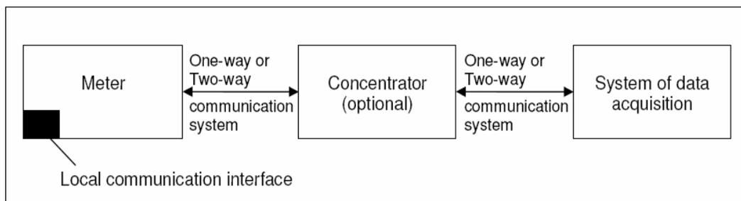
**Figure 2: General structure of a smart metering system** (Source: Figure 6, ERGEG Status Review of Regulatory Aspects of Smart Metering<sup>6</sup>)
